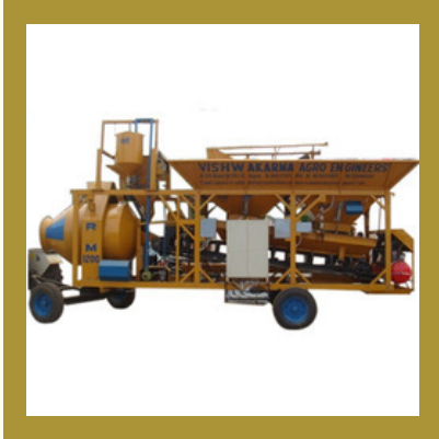
Automatic Batching Plant Conveyor
